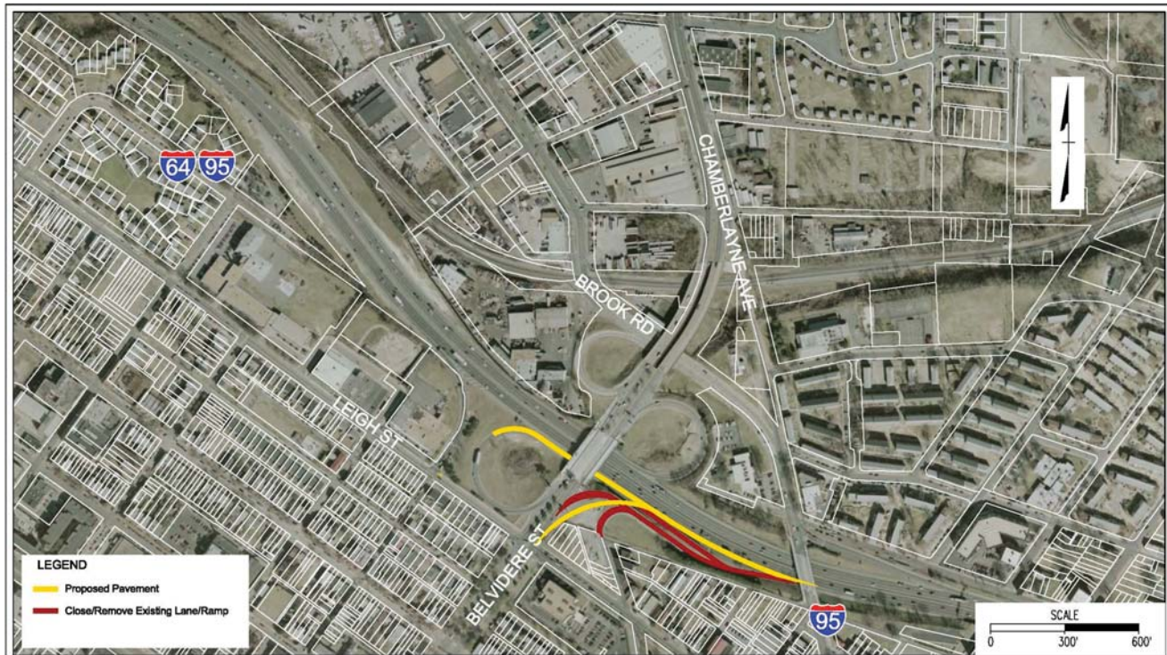
Figure 43: SYIP #4 - Belvidere Street Interchange Improvements
